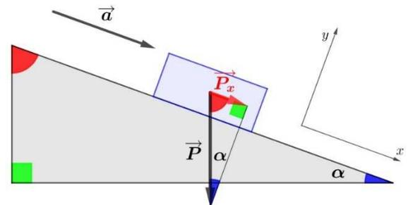
$$P \sin \alpha = ma \quad \Rightarrow \quad mg \sin \alpha = m \frac{v_1}{t_1} \quad \Rightarrow \quad \sin \alpha = \frac{v_1}{gt_1} \quad \Rightarrow \quad \alpha = \sin^{-1} \frac{v_1}{gt_1} = \mathbf{4,7^\circ}$$
