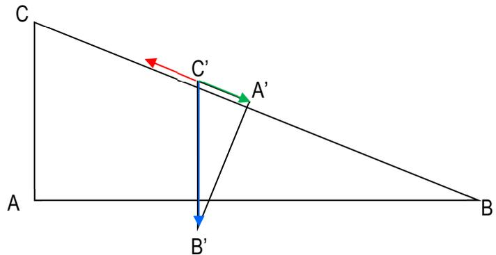
$$F = 35,0 \text{ kg} \cdot 9,81 \text{ m/s}^2 \cdot \frac{1,80 \text{ m}}{3,70 \text{ m}} = 167 \text{ N}$$
